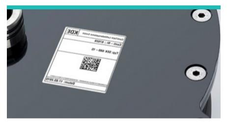
"Each system's DataMatrix barcode contains both the serialised GTIN for the whole system as well as the serialised GTINs for the components in the system since markings or labels don't always adhere to some components such as rubber bellows," explains Neumann. "All serialised GTINs can now be easily captured with a single scan anywhere in our supply chain processes—manufacturing, maintenance and repair and overhaul cycles."
