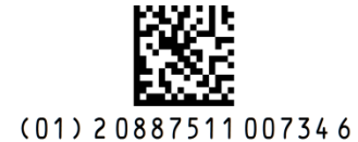
Figure 6d: GTIN-14 in a GS1 DataMatrix Barcode (DI only or PI can be added as shown in 6c)
