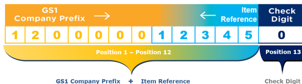
Figure 5-2: Segments of a GTIN-13 (based on the hypothetical GTIN “1200000123450”)
